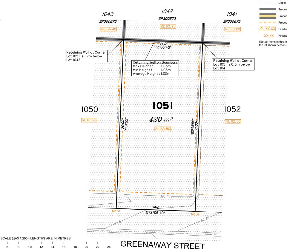
**Design Contours** - Depth of Fill Contours Proposed Retaining Wall TEVIOT Proposed Tiered Retaining Wall Proposed Earthworks Pad RL XX.XX Finished Pad Design Level XX.XX Finished Surface Design Level (Not all items in this legend may be relevant to
