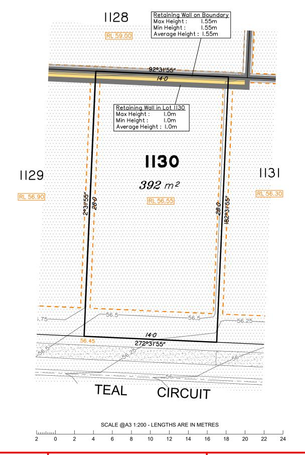
**LEGEND** Area of Fill Area of Cut **Design Contours** - Depth of Fill Contours Proposed Retaining Wall Proposed Tiered Retaining Wall - - - Proposed Earthworks Pad RL XX.XX Finished Pad Design Level XX.XX Finished Surface Design Level (Not all items in this legend may be relevant to
